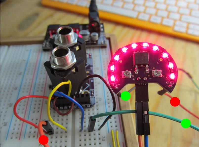
Assembled PCB in use with Jack Me Module. The green dots reflect SIG - (Shield/GND) and the red dots reflect SIG +.(Tip/Ring)
